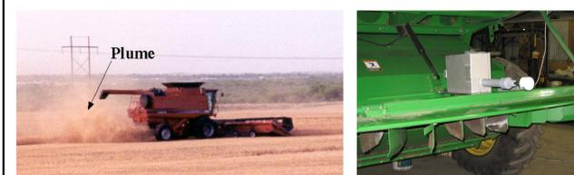
Image (left) showing the plume produced by a combine while harvesting wheat in North Dakota. Image (right) showing the exit of the chopper chute on the bullet rotor combine used for sampling with the six-channel particle counter. The rear-facing inlet samples aerosol concentrations at center of the airflow just outside the exit of the chute.
