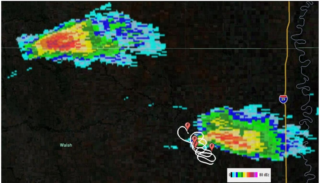
**Figure 3:** Google Earth image showing the aircraft flight track (white line) on 1 July 2008 from 23:30:44 and 23:41:40 UTC. The red balloons indicate the locations where each set of flares was lit. The color overlay is the level II radar reflectivity at the 0.5 elevation angle from the National Weather Service radar in Mayville, North Dakota.
