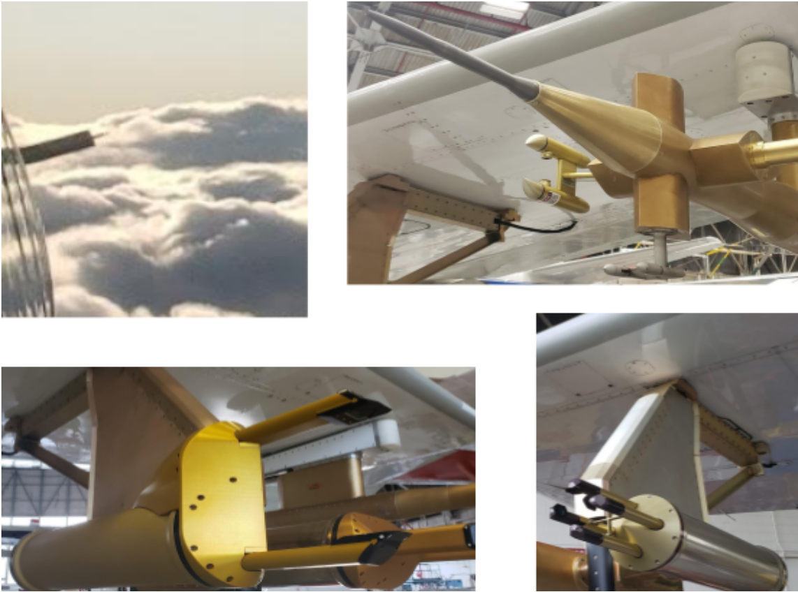
Figure 4: Instrument configuration of the UND Cloud Probes during IMPACTS 2020. The Rosemount Icing Detector (RICE Probe) is mounted on the fuselage on the starboard side of the forward portion of the aircraft (top left). Probes mounted on wing pylons include a Two-Dimensional Stereo (2D-S) probe (bottom right), two High Volume Precipitation Spectrometer Version 3 (HVPS-3) probes (bottom left), a King Liquid Water Sensor (King Probe), and a Cloud Droplet Probe (CDP), the latter two being mounted on the same boom (top right).
