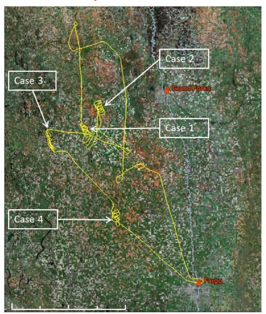
Flight track of the first flight conducted on 26 July 2012. The spirals are when samples were made at cloud base, while the long straight legs are transects between possible targets.
