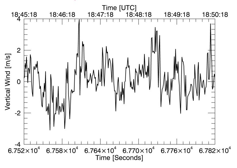
Vertical wind velocity measured by the Aircraft Integrated Meteorological Measurement System (AIMMS) during the first flight on 26 July 2012 flight over five minutes.
