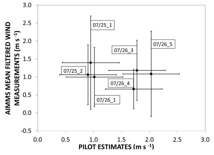
Horizontal bars represent  $\pm$  0.50 m s<sup>-1</sup> pilot uncertainty. Vertical error bars indicate  $\pm$  one standard deviation for the AIMMS 1 Hz measurements obtained over five minutes. Boxes denotes the flight date and corresponding case number. Three points (07/25 1&2, and 07/26 4) have been offset for visual clarity of error bars.
