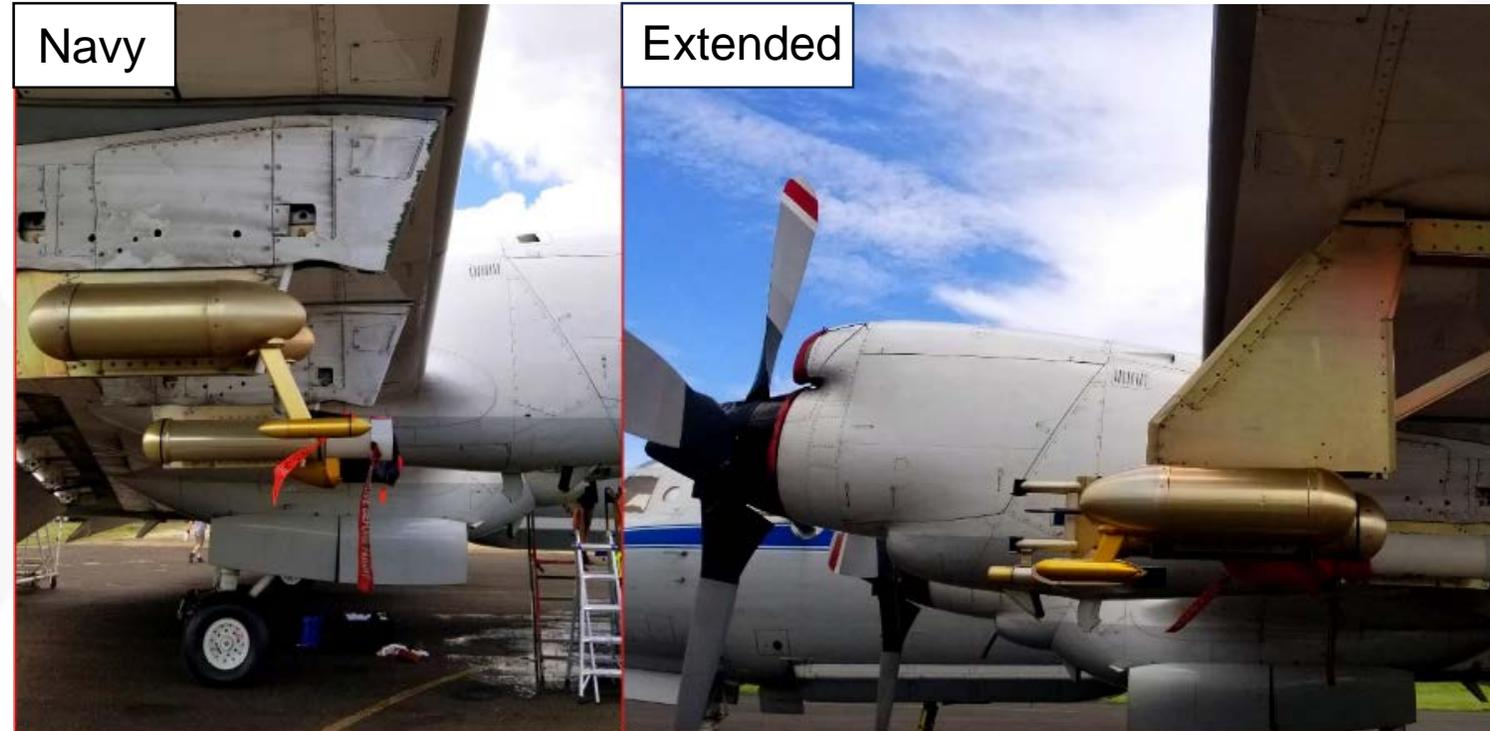
Navy - NASA P-3 Original Pylon Configuration
