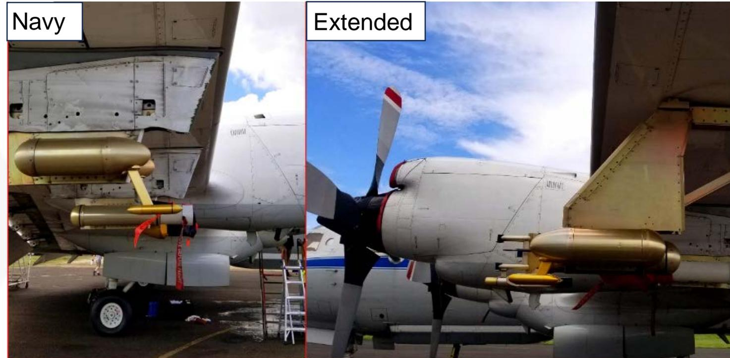
Navy - NASA P-3 Original Pylon Configuration
