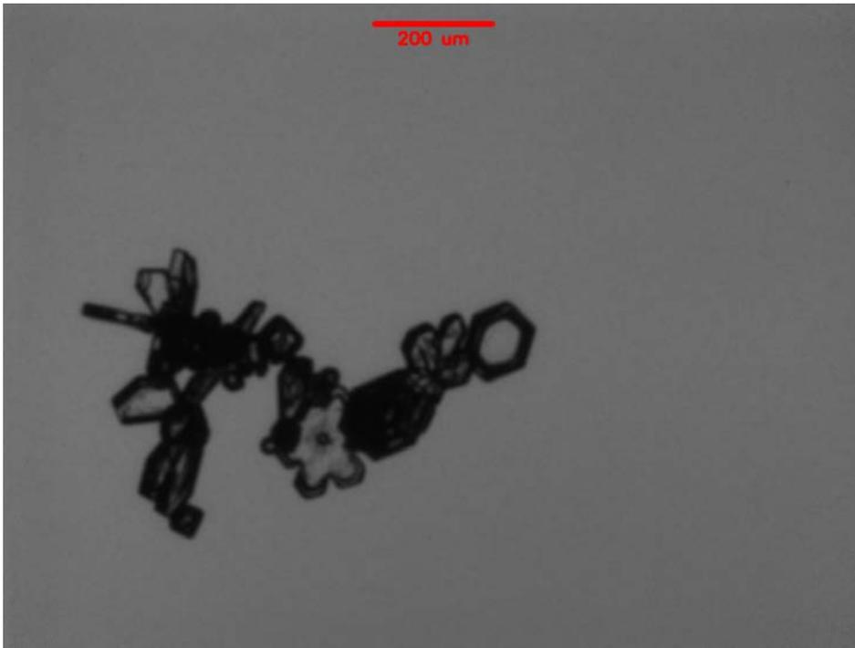
Figure 1. Image of a chain aggregate taken by the Particle Habit Imaging and Polar Scattering (PHIPS) probe on 3 August 2019 at 16:05:34 UTC.
