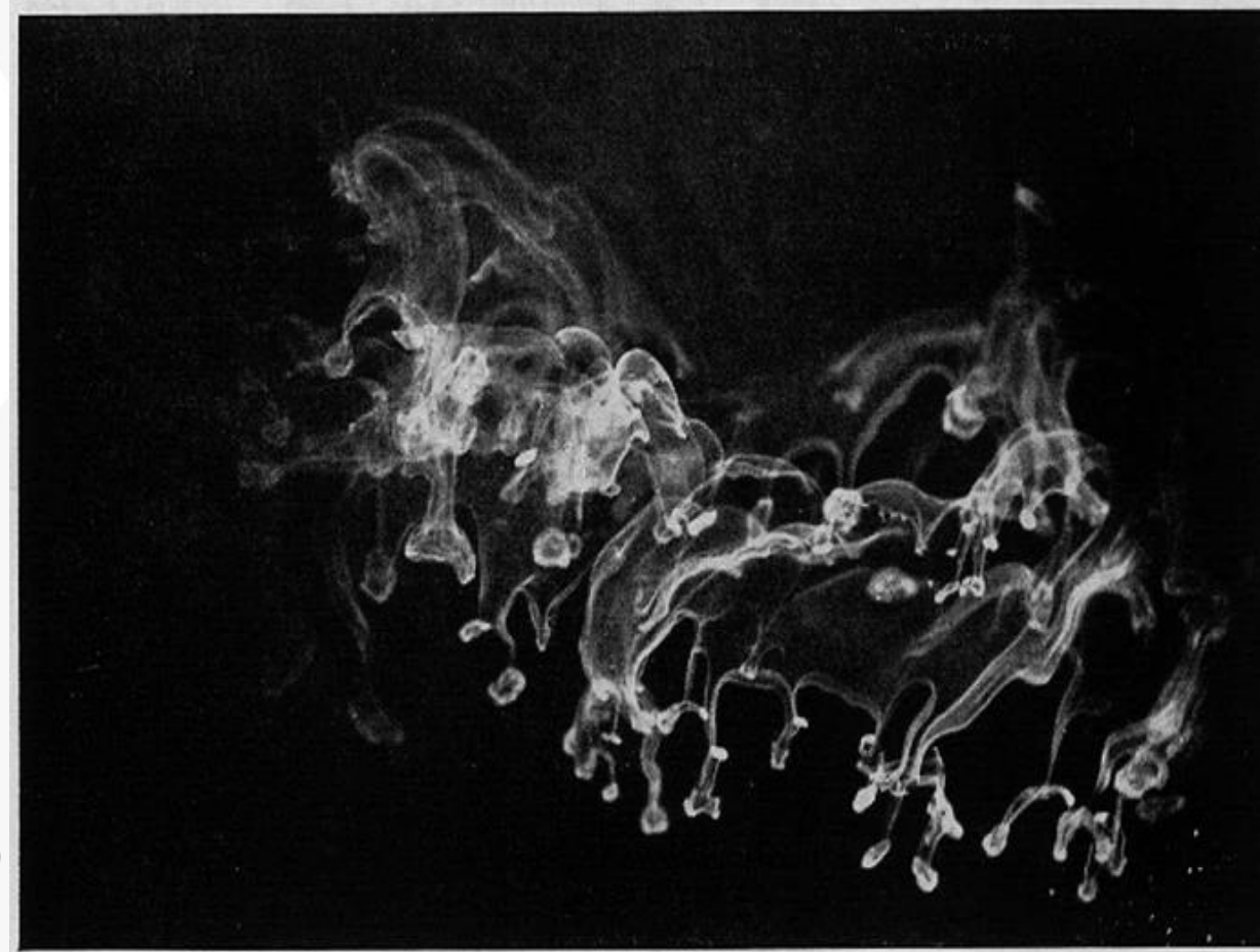
Schaefer 1948. Trail of ice crystals produced in cold chamber by seeding with a needle cooled below -39 °C
