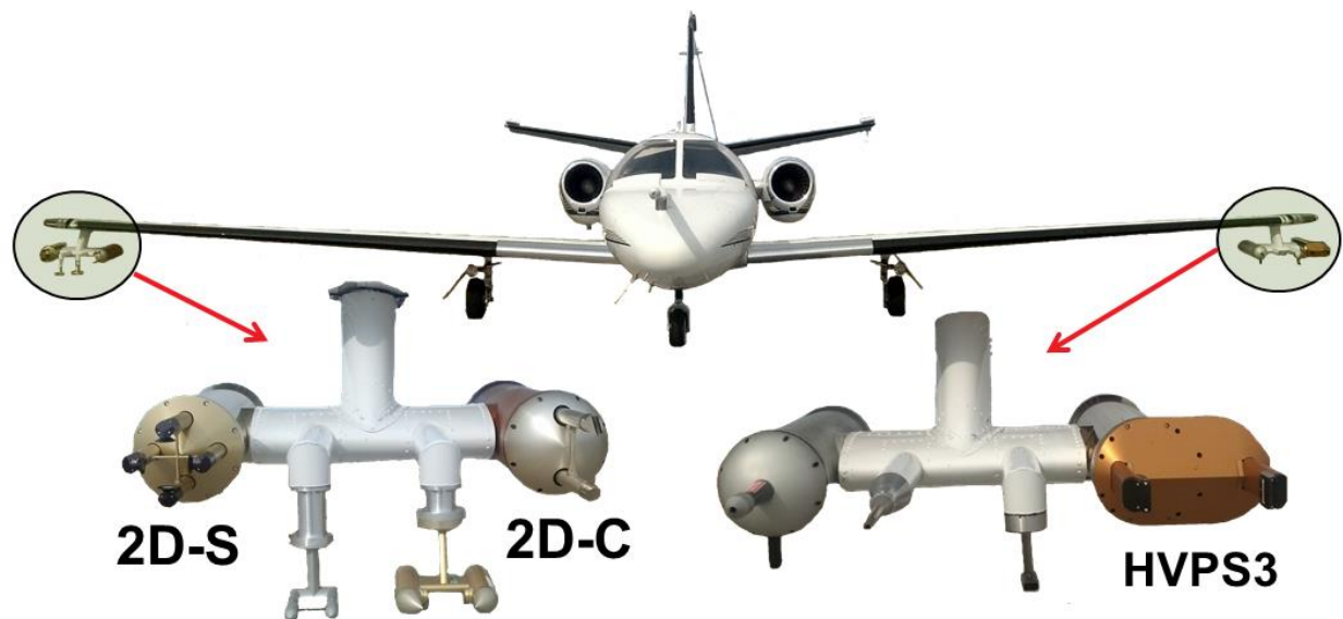
Figure 1: Schematic showing images of the Two-Dimensional Optical Array Cloud (2D-C) Probe, Two-Dimensional Stereo (2D-S) Probe, and High Volume Precipitation Spectrometer Version 3 (HVPS3) mounted on the University of North Dakota Citation II Research Aircraft. Additional probes are shown and mounted on the aircraft but are not highlighted.
