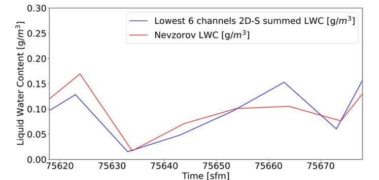
Liquid water content (LWC) for Nevzorov probe compared to 2D-S mass (top) and a time series of the lowest six channels of 2D-S LWC compared to Nevzorov LWC (bottom).
