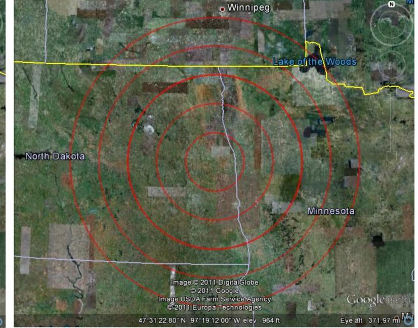
Research Aircraft's flight track. The flight track Research Aircraft's flight track. The flight track is based on 1 Hz GPS data that has been is based on 1 Hz GPS data that has been automatically processed to create a kml automatically processed to create a kml
