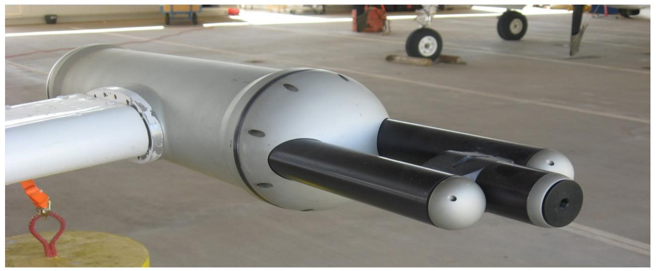
This FSSP-100 has the Signal Processing Package (SPP) upgrade to the FSSP-100 probe. This package replaces original PMS electronics with modern high-speed circuitry.
