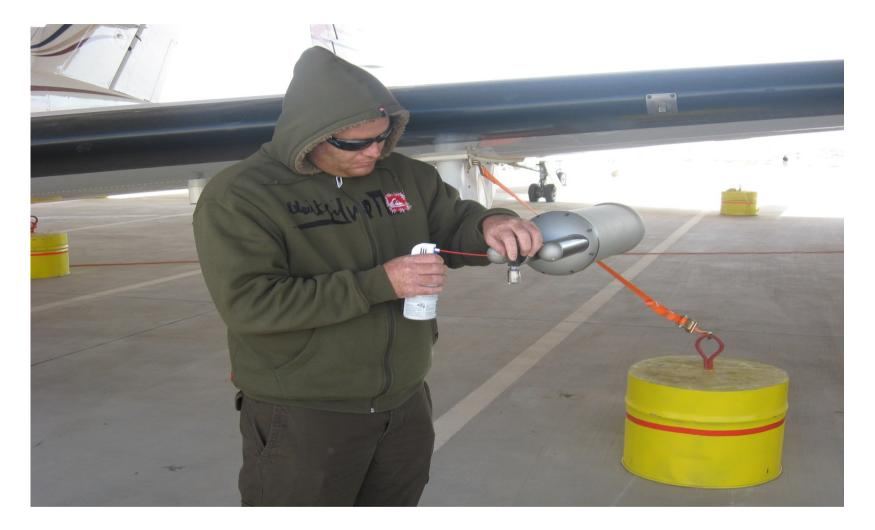
The FSSP is calibrated to determine the instruments depth of field, laser beam diameter, and channel size boundaries. The channel counts obtained from measurements on beads of known size are used to determine the FSSP channel boundaries.
