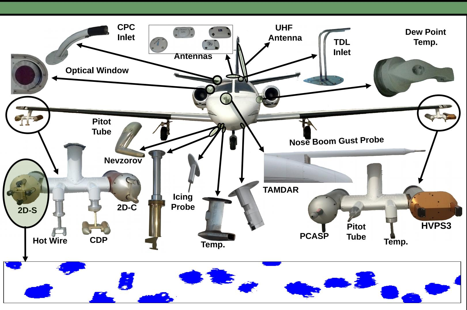
Citation Research Aircraft for the CAPE2015 field project conducted to sample Florida thunderstorm anvils. An example image buffer is shown for the 2D-S, where the top to bottom length is 1,280 µm, corresponding to 128 diode of 10 µm each.
