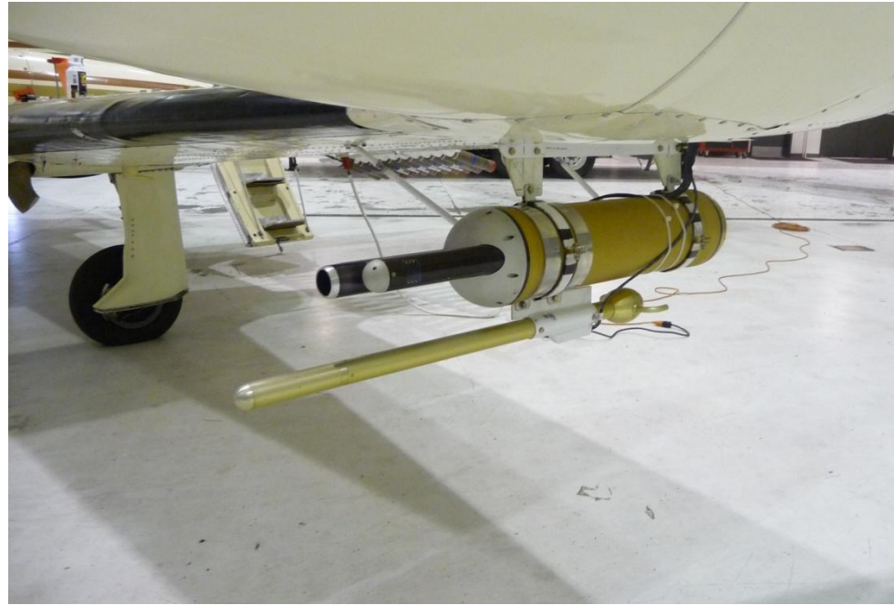
Aircraft Integrated Meteorological Measurement System (AIMMS) under the left wing on the Cessna 340 (ND98585) used during the 2012 POLCAST4 field project.
