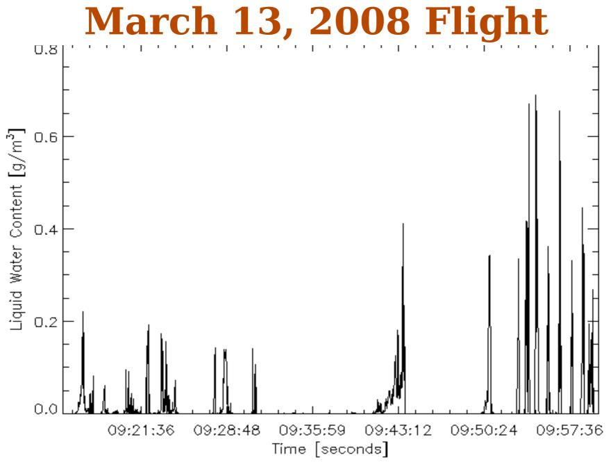
FSSP cloud liquid water content measurements near Hail, Saudi Arabia at -16 C and 19,000 ft.
