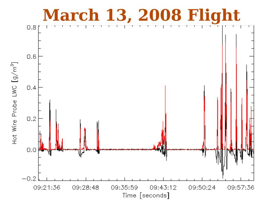
Hot Wire Probe (Black) and FSSP (red) cloud liquid water content measurements near Hail, Saudi Arabia at -16 C and 19,000 ft.
