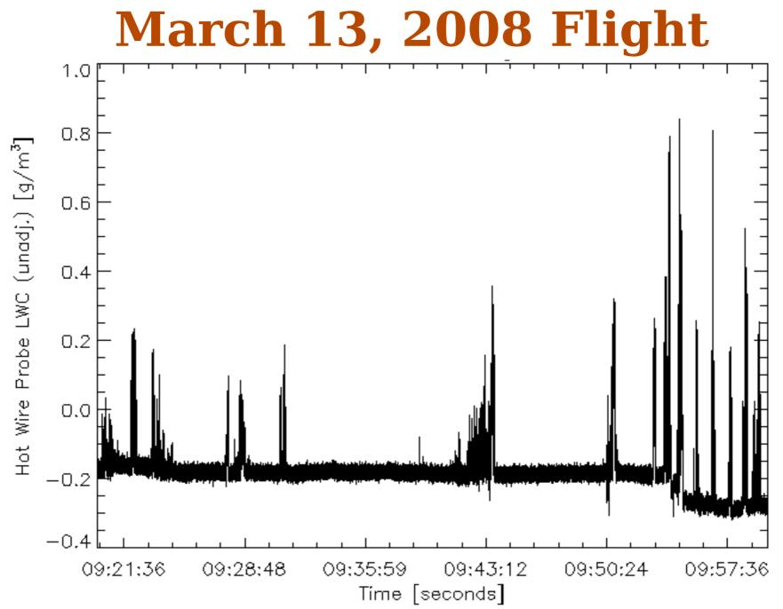
Hot Wire Probe cloud liquid water content (unadjusted offset) measurements near Hail, Saudi Arabia at -16 C and 19,000 ft.
