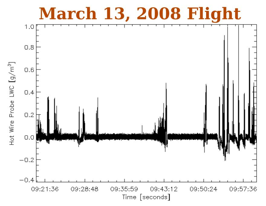
Hot Wire Probe cloud liquid water content (adjusted offset) measurements near Hail, Saudi Arabia at -16 C and 19,000 ft.
