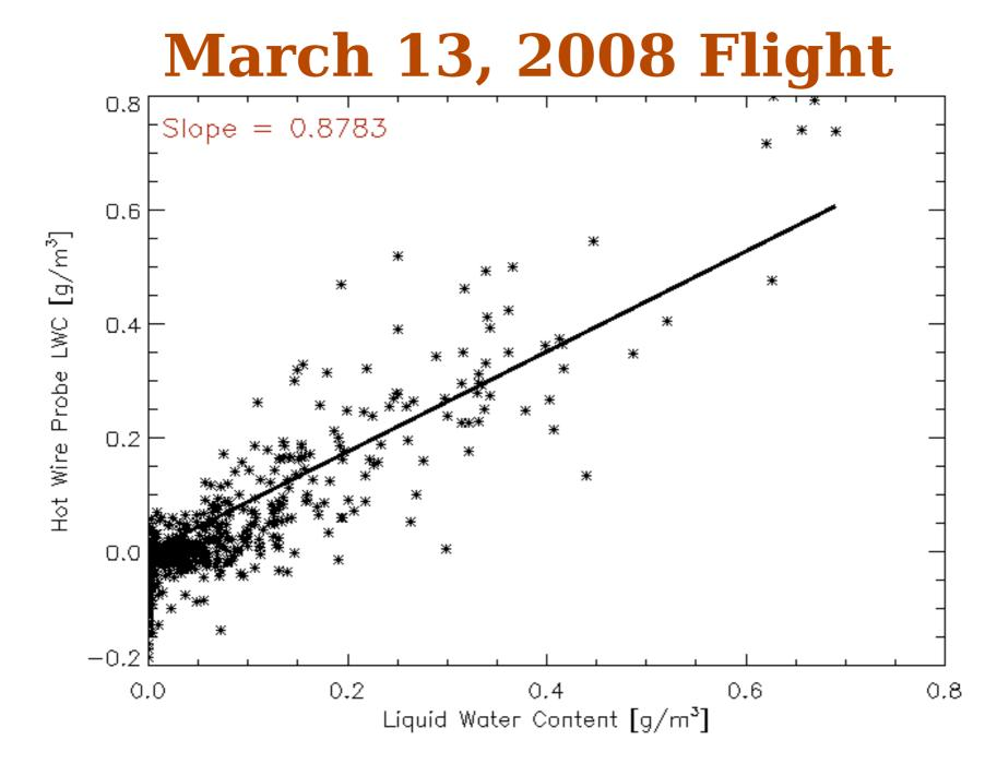
FSSP cloud liquid water content versus the Hot Wire Probe cloud liquid water content measurements between 9:20 and 10:00.
