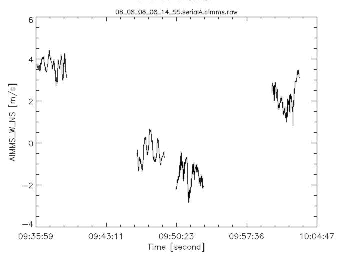
The north/south component of the horizontal winds from the AIMMS probe on August 8, 2008. The first and last intervals are when the aircraft is heading north, the two intervals in the middle are when the aircraft is heading south.
