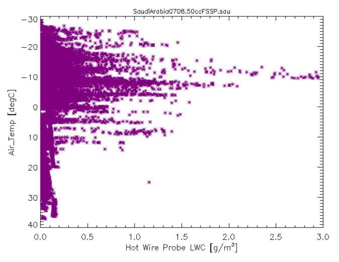
The 1 Hz liquid water from the DMT hot wire probe for all January-April 2008 Saudi Arabia flights measurements with FSSP total concentrations above 50 # cm<sup>-3</sup>.
