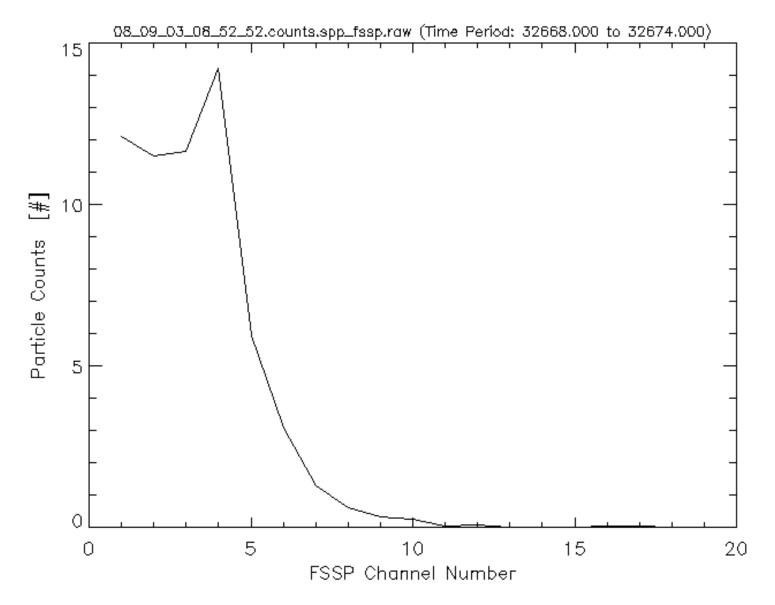
September 3, 2008 calibration check on the NCAR FSSP (SN 277-0676-06) using 15  $\mu m$  beads. Calibration check was preformed while the probe was in Saudi Arabia on the Research
