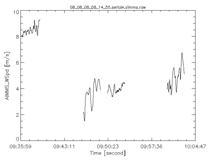
The magnitude of the horizontal winds from the AIMMS probe on August 8, 2008. The first and last intervals are when the aircraft is heading north, the two intervals in the middle are when the aircraft is heading south.
