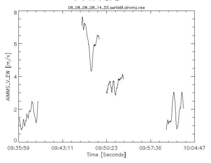
The east/west component of the horizontal winds from the AIMMS probe on August 8, 2008. The first and last intervals are when the aircraft is heading north, the two intervals in the middle are when the aircraft is heading south.
