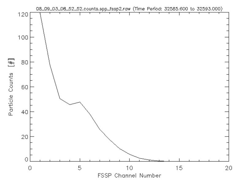
September 3, 2008 calibration check on the WMI FSSP (SN 1947-0281-60) using 15 µm beads. Calibration check was preformed while the probe was in Saudi Arabia on the Research
