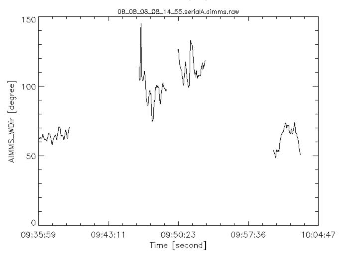
The direction of the horizontal winds from the AIMMS probe on August 8, 2008. The first and last intervals are when the aircraft is heading north, the two intervals in the middle are when the aircraft is heading south.
