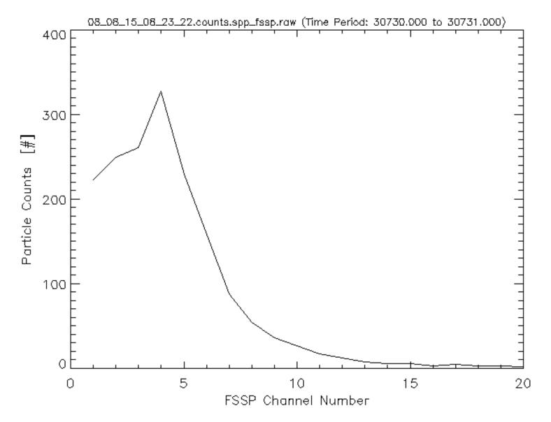
August 15, 2008 calibration check on the WMI FSSP (SN 1947-0281-60) using 15 μm beads. Calibration check was preformed while the probe was in Saudi Arabia on the Research
