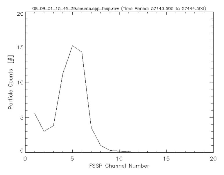
August 1, 2008 calibration check on the NCAR FSSP (SN 277-0676-06) using 15  $\mu$ m beads. Calibration check was performed at UND before being shipped to Saudi Arabia.
