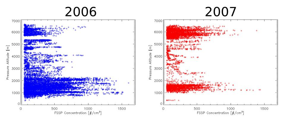
The 1 Hz cloud droplet concentration at standard temperature and pressure versus pressure altitude for all Mali 2006 (Top-Blue) and Mali 2007 (Bottom-Red) measurements with concentrations above 50 # cm-3.
