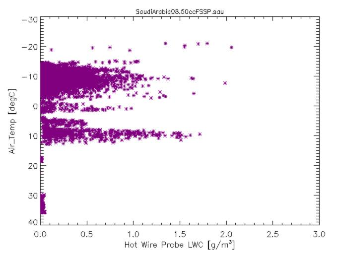
The 1 Hz liquid water from the DMT hot wire probe for all June and July 2008 Saudi Arabia flights measurements with FSSP total concentrations above 50 # cm<sup>-3</sup>.
