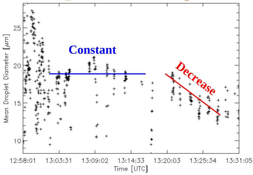
Time series of mean droplet diameter (1 Hz data) at 18,000 ft measured by an FSSP on the 9 April 2009 Saudi Arabia flight.
