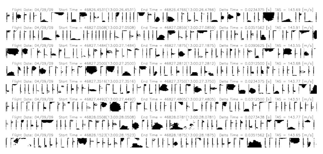
Images from the 2-DC between 13:00:26.45 and 13:00:28.19 (less than 2 seconds total) which correspond to the maximum liquid water content equivalent (1 Hz data) measured by 2-DC probe between on 9 April 2009 research flight in Saudi Arabia.
