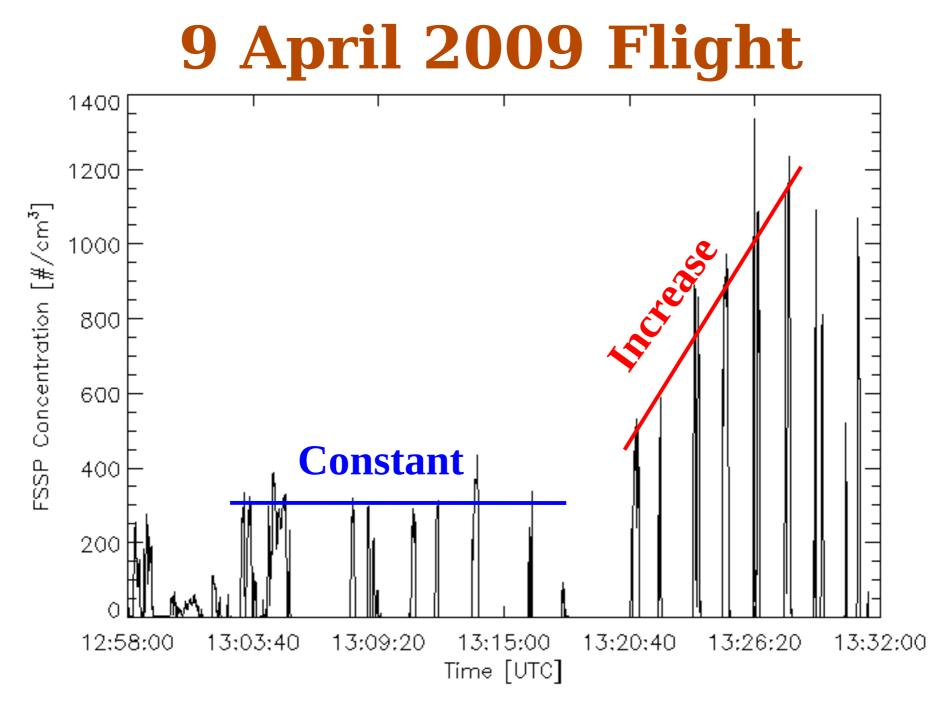
Time serial of cloud droplet concentration (1 Hz average) at 18,000 ft measured by an FSSP on the 9 April 2009 Saudi Arabia flight.
