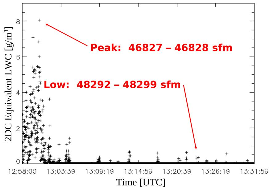
Liquid water content equivalent (1 Hz data) at 18,000 ft measured by 2-DC probe on a research flight in Saudi Arabia.
