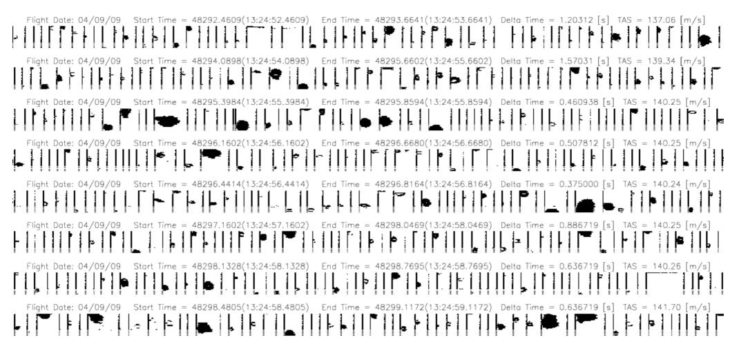
Images from the 2-DC between 13:24:52.46 and 13:24.59 (9 seconds total) which correspond to the low liquid water content equivalent (1 Hz data) measured by 2-DC probe on 9 April 2009 research flight in Saudi Arabia.
