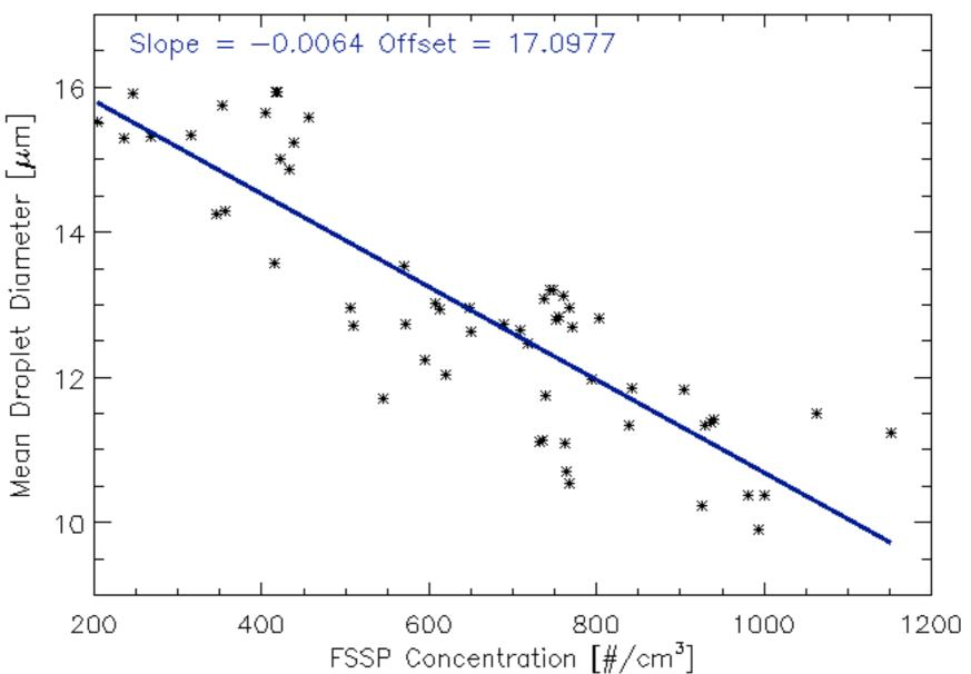
Only 1 Hz measurements with DMT Hot Wire liquid water content above  $1.0 \text{ g/m}^3$  are included.
