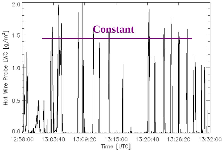
Liquid water content at 1 Hz measured by a DMT Hot Wire Probe on the 9 April 2009 research flight in Saudi Arabia.
