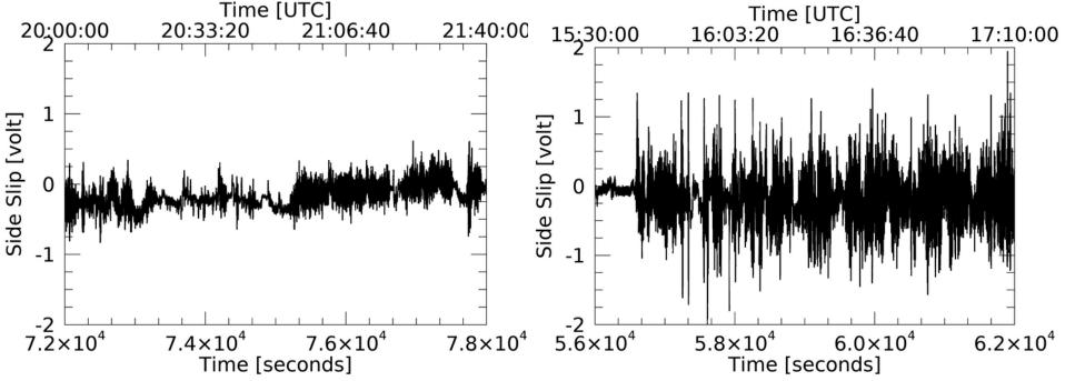
Time series (25 Hz) of voltage from the side slip pressure transducer on the North Dakota Citation Research Aircraft during research flights. The same data system and analogto-digital board is used on both flights.
