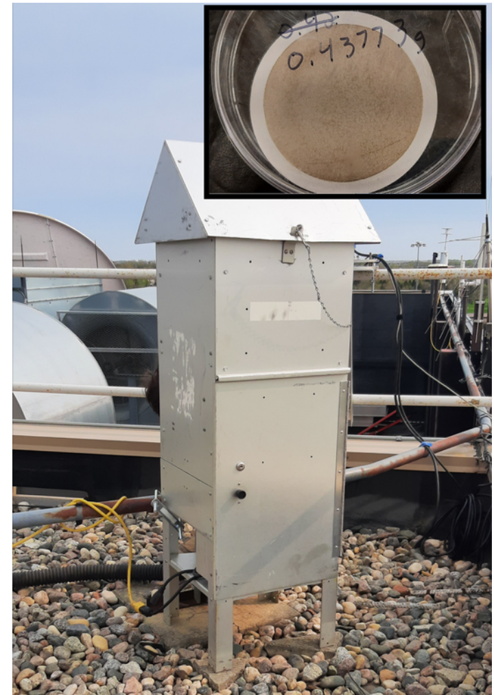
Image showing a high volume filter sampler on top of Clifford Hall and a filter sample obtained with the sampler.
