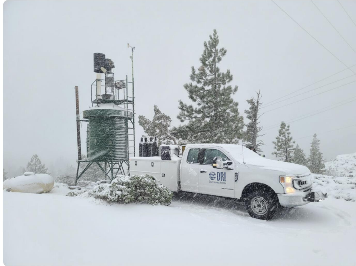
Above: A DRI cloud-seeding generator and maintenance truck in a wintery, mountain-top setting. Credit: Jesse Juchtzer/DRI
