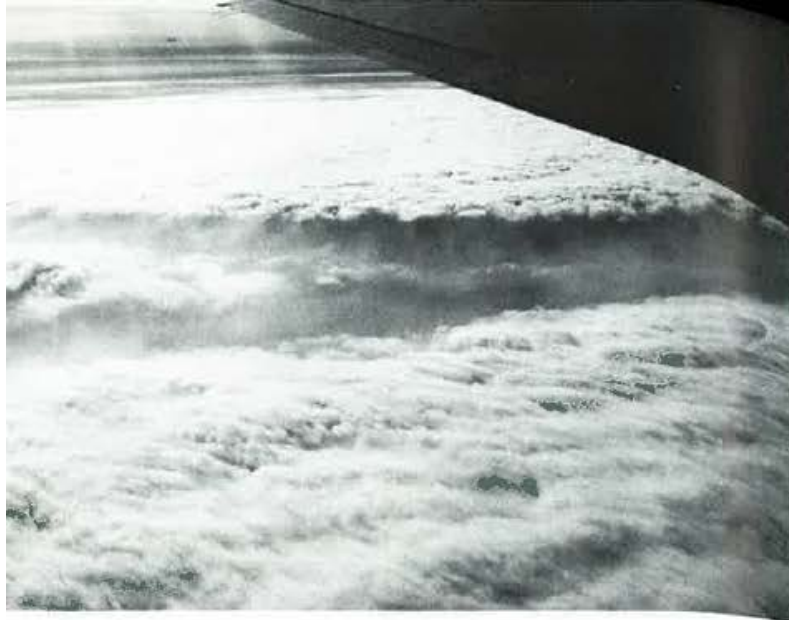
Pl.259 Two lines cut through a deck of supercooled clouds, using dry ice fragments dispensed at rate of about 1 kg/km. Thin veils of ice crystals remain in seeded area but most have fallen.
