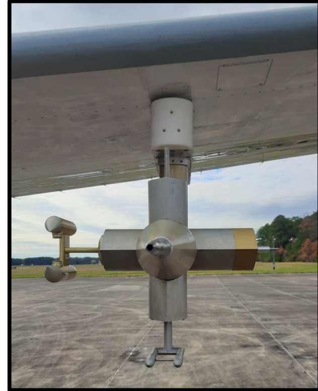
Rosemount Icing Detector probes on the fuselage and on hot-wire boom under the left wing of P-3 aircraft for NASA IMPACTS 2023 field project.
