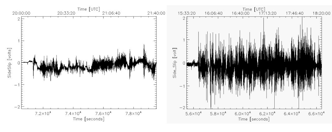
Voltage measurement from the side slip pressure transducer on the North Dakota Citation Research Aircraft.
