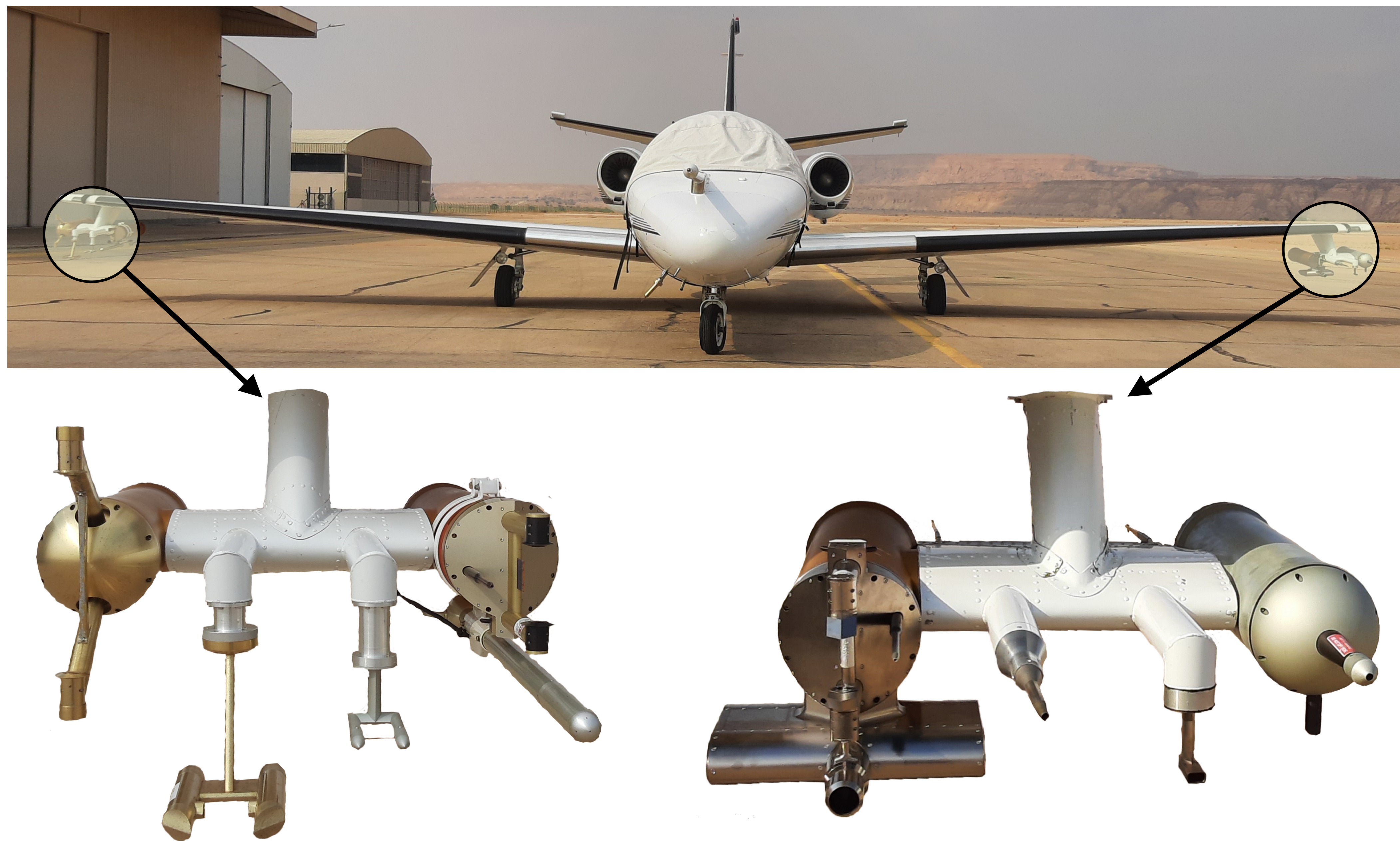
Image showing the aircraft instruments deployed on the North Dakota Citation Research Aircraft, which included a Cloud Droplet Probe (CDP).
