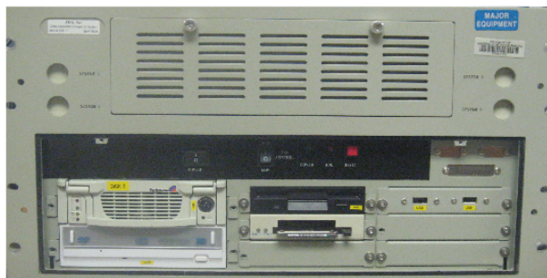
Fig. 1 Science Engineering Associates, Inc. model M300 Data Acquisition System used for aircraft field projects at the University of North Dakota.
