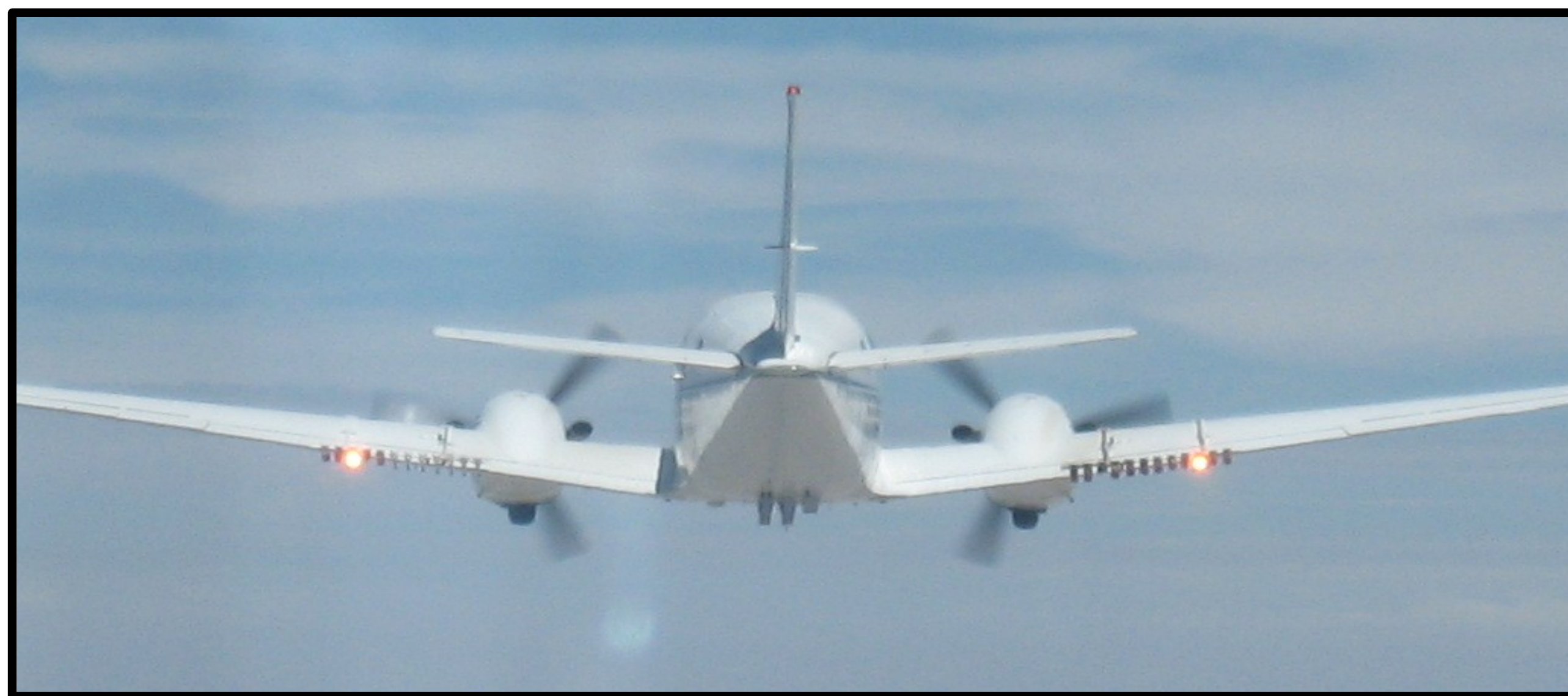
King Air CJ-90 Aircraft with hygroscopic flares lit.
