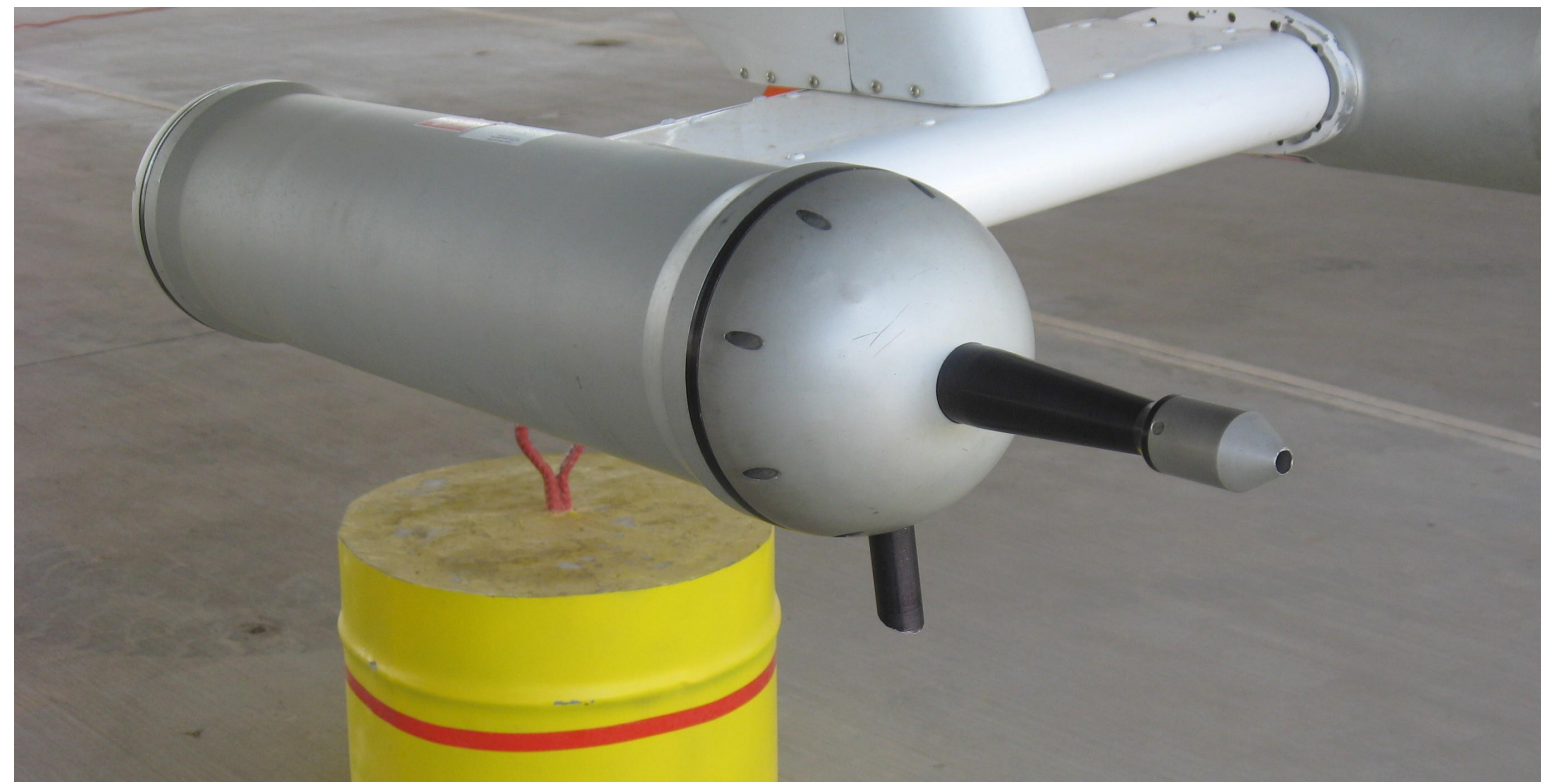
PCASP instrument used in Mali
